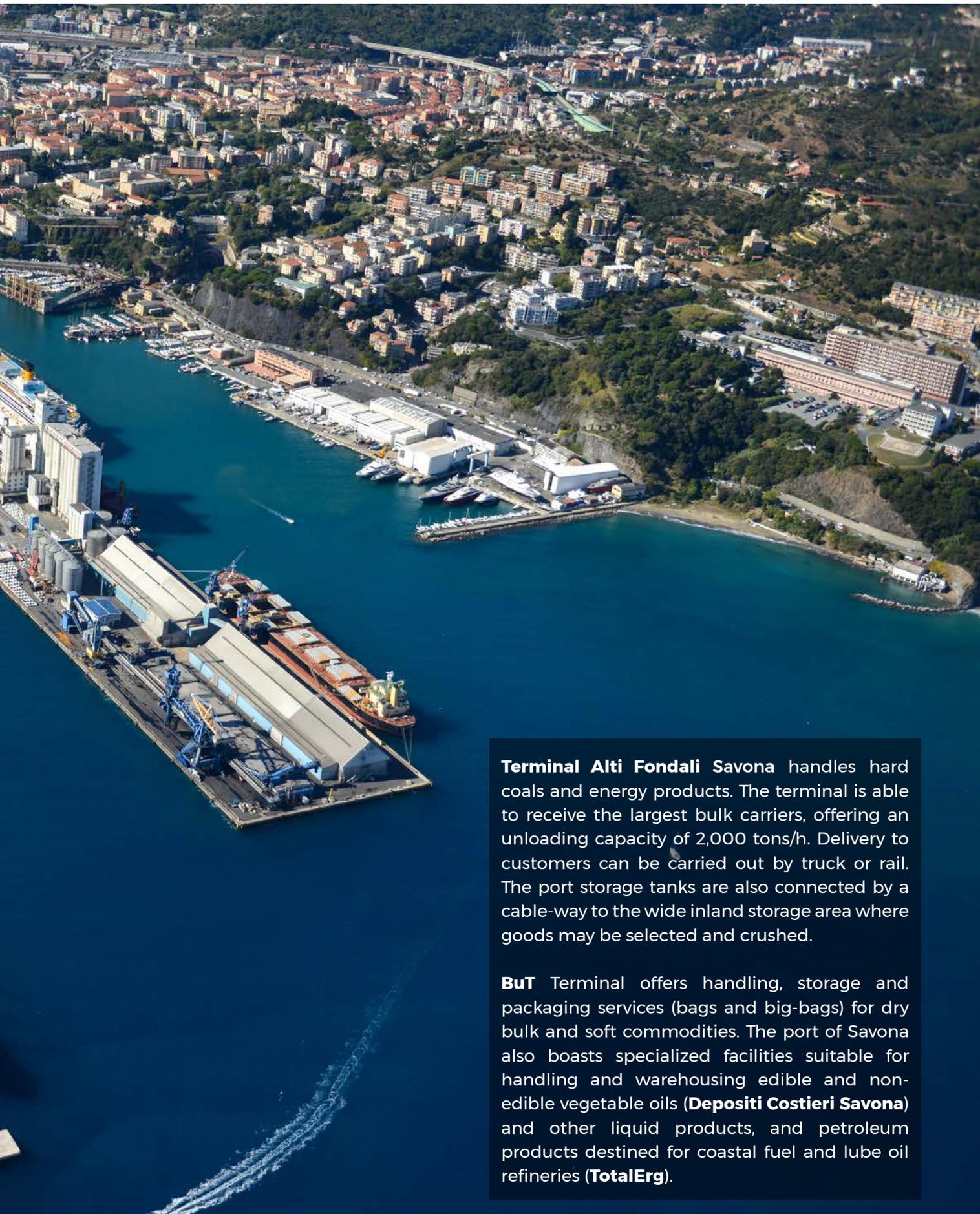
**Terminal Alti Fondali Savona** handles hard coals and energy products. The terminal is able to receive the largest bulk carriers, offering an unloading capacity of 2,000 tons/h. Delivery to customers can be carried out by truck or rail. The port storage tanks are also connected by a cable-way to the wide inland storage area where goods may be selected and crushed.
